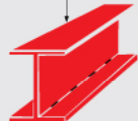
H-beam Assembling (By Auto Spot Welding)
