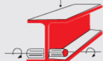
H-beam Fabrication straightening (By submerge arc welding)
